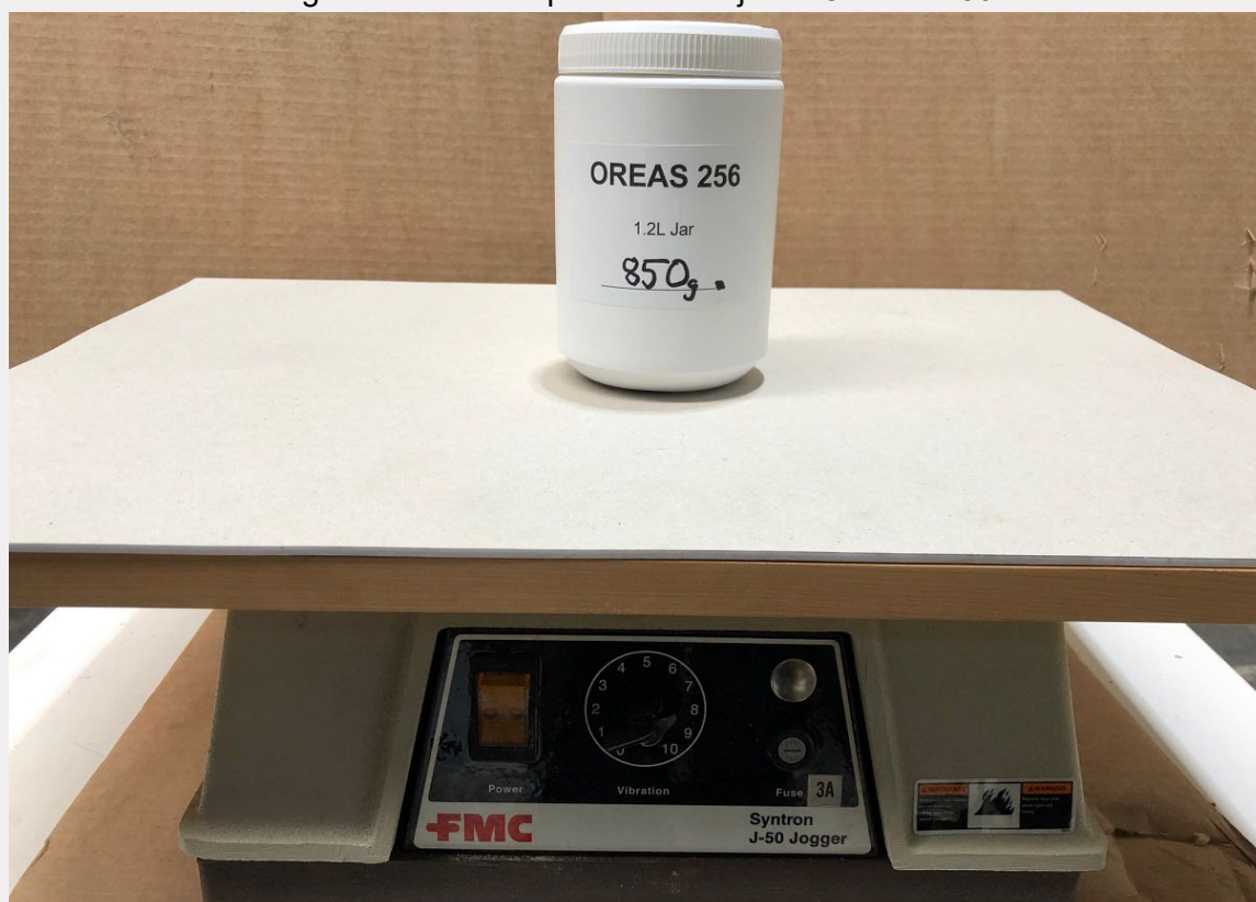
Figure 1. Vibration platform with jar of OREAS 256.
