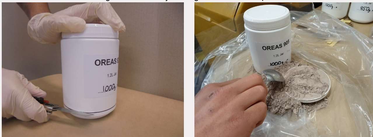
Figure 2. Base of jar being cut and subsampled.
